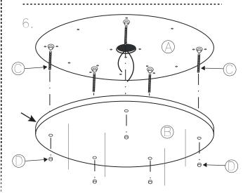
Remove rods and attach  $\bigcirc$  to  $\bigcirc$  with the button head screws  $\bigcirc$
